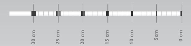
**NOTE:** The actual cm length is the middle of the marking: the middle black dash for the odd numbers or the space between the middle black dashes for the even numbers.
