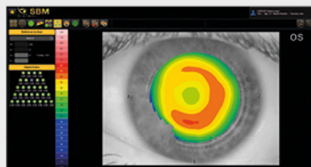
Advanced altimetry A differential altimetry map between a reference surface and the patient's eye decomposed in Zernike polynomials up to 7th order.
